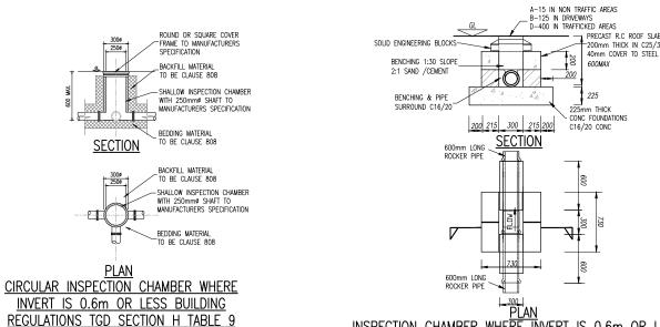
INSPECTION CHAMBER WHERE INVERT IS 0.6m OR LESS BUILDING REGULATIONS TGD SECTION H TABLE 9
